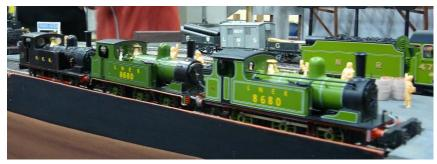
**PHOTO:** CME Wilson Worsdell's J72 (NER Class E1) 0-6-0 tank engines. A total of 113 J72s were built in nine batches from 1898 and 1951. This large separation in time (53 years) between the construction of the first and last J72s, is probably a record for a British steam locomotive class. The J72s proved very successful and would eventually be found throughout the LNER system. They were the only class that was allocated to all of the LNER's major constituent companies.
